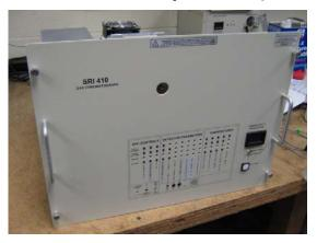
Both configurations include two FID detectors. FID#1 speciates the sample into methane, ethane, propane, iso and normal butane, iso and normal pentane
